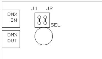
Two optional jumpers allow configuration of the 3008R relay card..
